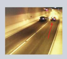
ClearWay detects and tracks the two vehicles despite the thick smoke in the tunnel. The whole event was recorded automatically for ease of post-event analysis.
