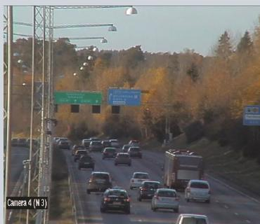
Radar detects a stopped vehicle during heavy traffic. The nearest camera is redirected to provide a visual giving the operator more information about the event
