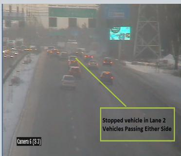
ClearWay detects a stopped vehicle. The radar software generates an alarm and directs the camera to the incident. The poor weather reduces the image quality, however, the radar still detects the event.
